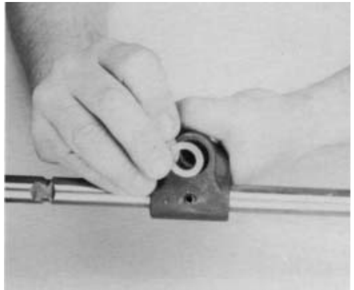
19. Remove the reverse plunger washer.
