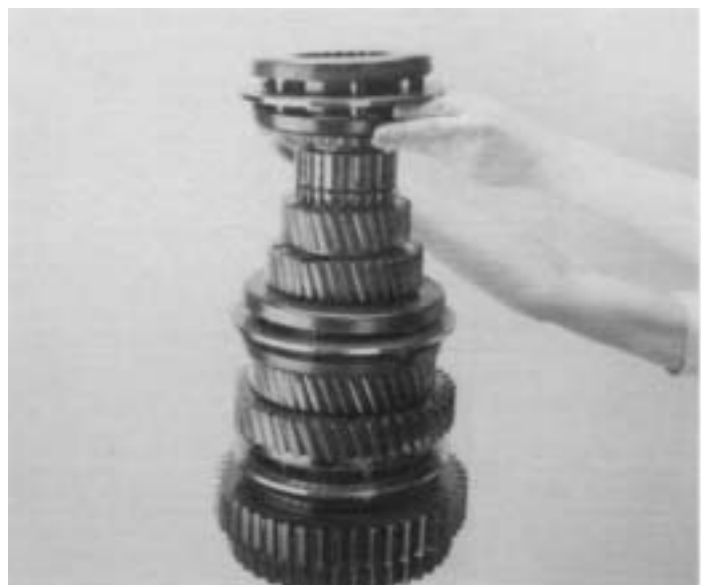
19. Lubricate and install the 5th-6th speed synchronizer cups and synchronizer ring identified FRONT facing up.
