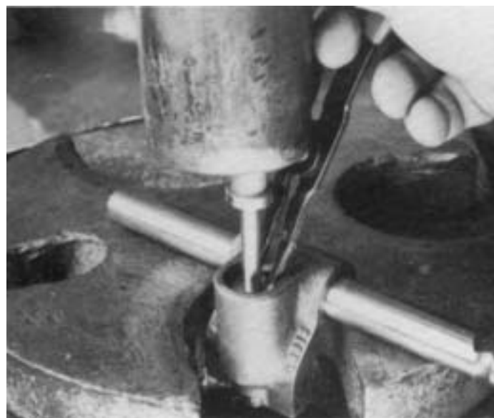
11. Place the shift yoke in a hand press. Depress retaining washer and spring and install the snap ring.
