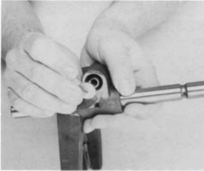
5. Install neutral retaining washer.
