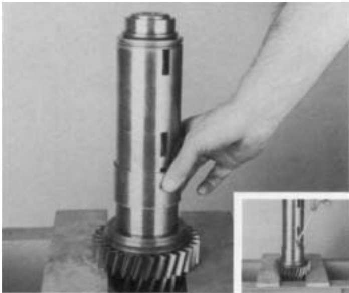
16. Remove the 5th speed gear key from shaft (inset). Using the rear face of 4th speed gear as a base, press it from the countershaft.
