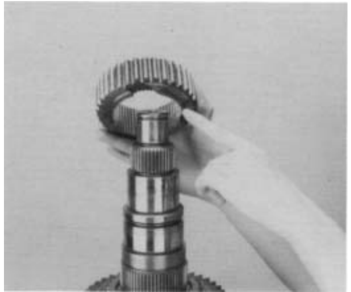
11. Lubricate the 3rd-4th speed shift hub and install the shift hub on the mainshaft splines with the flat side of the shift hub facing up.
