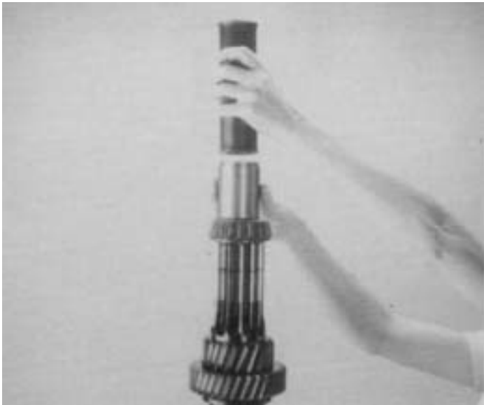
7. Using the proper size bearing driver, install the countershaft rear bearing on the countershaft rear. Make sure the bearing is seated against the countershaft.
